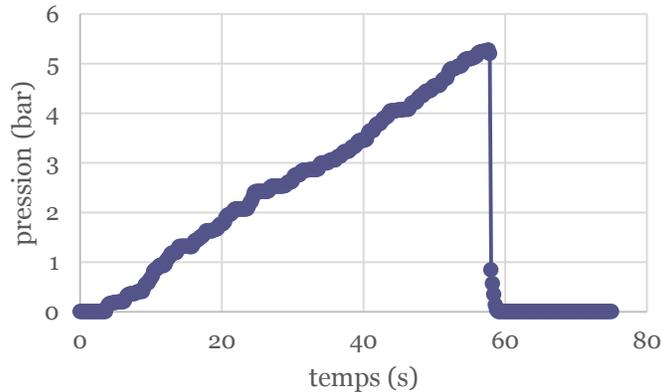
In free cell configuration the cell inflates without external constraints and strong peeling forces appear on the aluminum foil sealing line. At blow out, the sealing line opens quickly on one side of the cell and debonding of the seal spreads on several centimeter, leading to large opening of one side on complete leakage of components.
