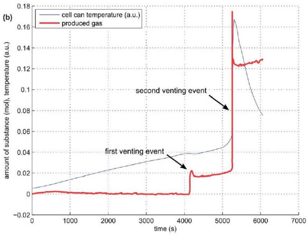
These curves clearly highlight the dependence between gas evolution and cell temperature. One evident strategy to prevent thermal runaway is to allow gas exhaust and then limit cell pressure build up and
