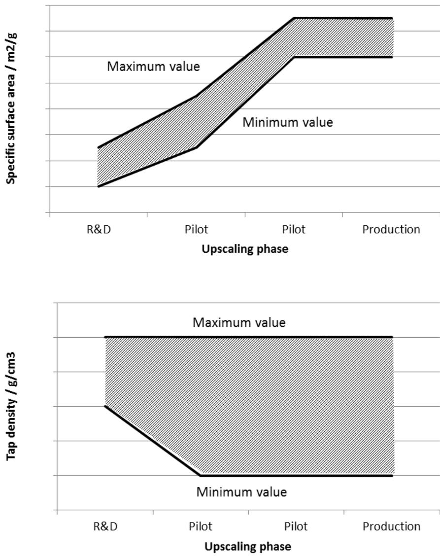
Figure 3 Evolution of Specific surface area and Tap density during upscaling
