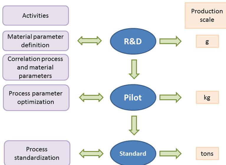
**Figure 1** Scheme reporting the typical upscaling procedure
