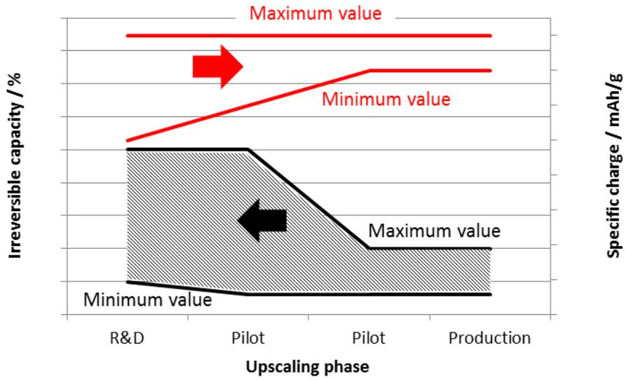
Figure 4 Evolution of the desired specific capacity and irreversible capacity during the upscaling activity
